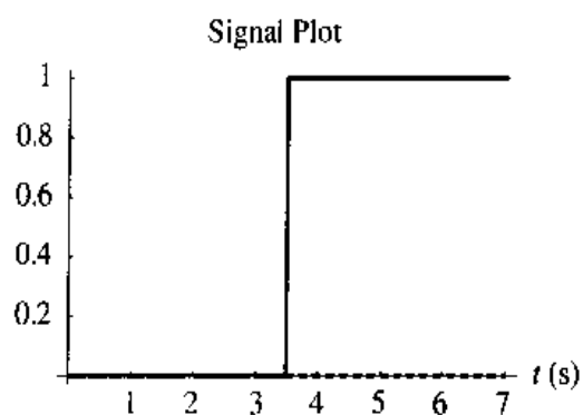
Figure 1.22 The continuous unit step signal, u(t) .
